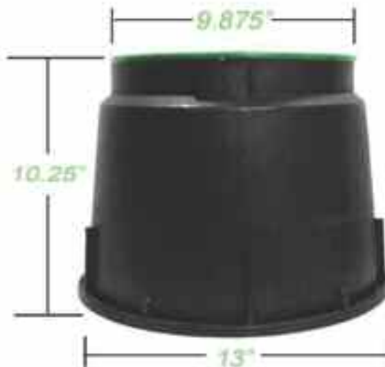
10" Round Valve Box: PART # 100 Black Body, Green Lid 100 Dimensions: Depth (Height): 10.25"; Lid: 9.875" Round; Inside Base Diameter: 11.5"; Outside Base Diameter: 13" 9 units per box. 120 units per pallet.
